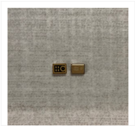
MEMS BOTTOM PORT DIGITAL MICROPHONE
