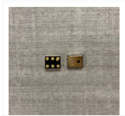
MEMS TOP PORT DIGITAL MICROPHONE
