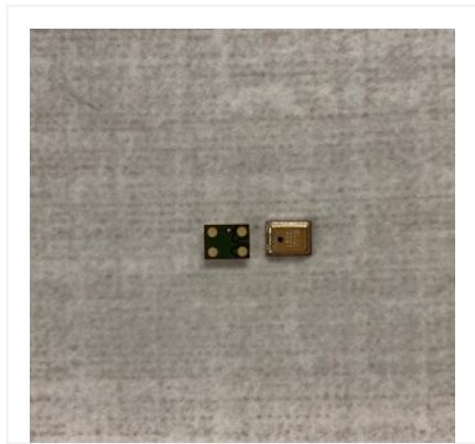
MEMS TOP PORT ANALOG MICROPHONE
