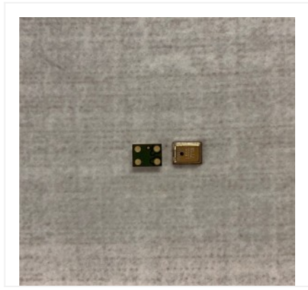
MEMS TOP PORT ANALOG MICROPHONE
