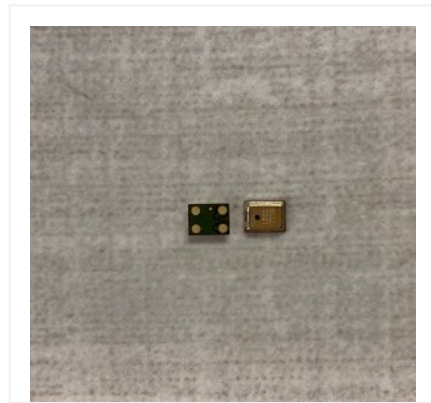
MEMS TOP PORT ANALOG MICROPHONE
