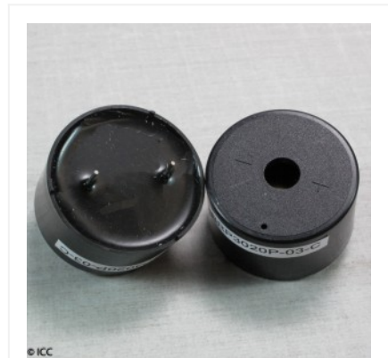
PIEZO ELECTRIC ALARM WITH INTERNAL CIRCUITRY
