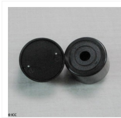
PIEZO ELECTRIC ALARM WITH INTERNAL CIRCUITRY
