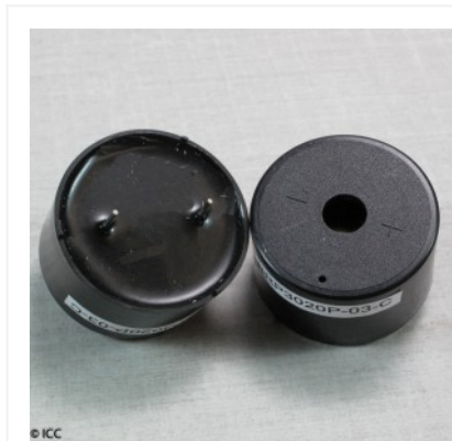
PIEZO ELECTRIC ALARM WITH INTERNAL CIRCUITRY
